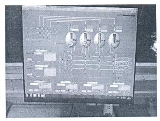
Automation is introduced at various stages like milk storage in silos: centralized monitoring and control of all pasteurizers (maintained exactly at required levels and ensures proper pasteurization). Milk silos are connected with the quality control laboratory for online approval process.
